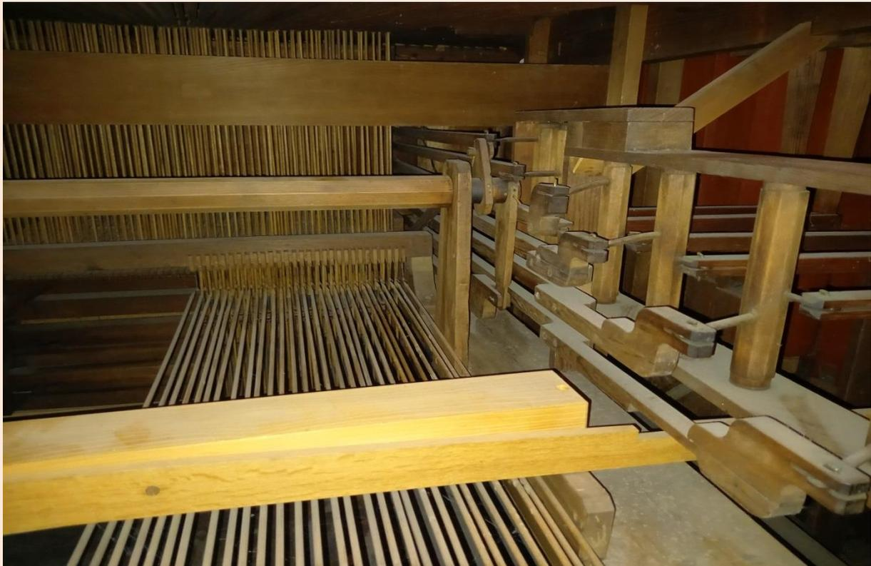
The key- and stop action is traditional made with wooden rollers and frames, trackers and metal arms and metal wiring. The nuts are from leather, pivot points are partly provided with cloth.
